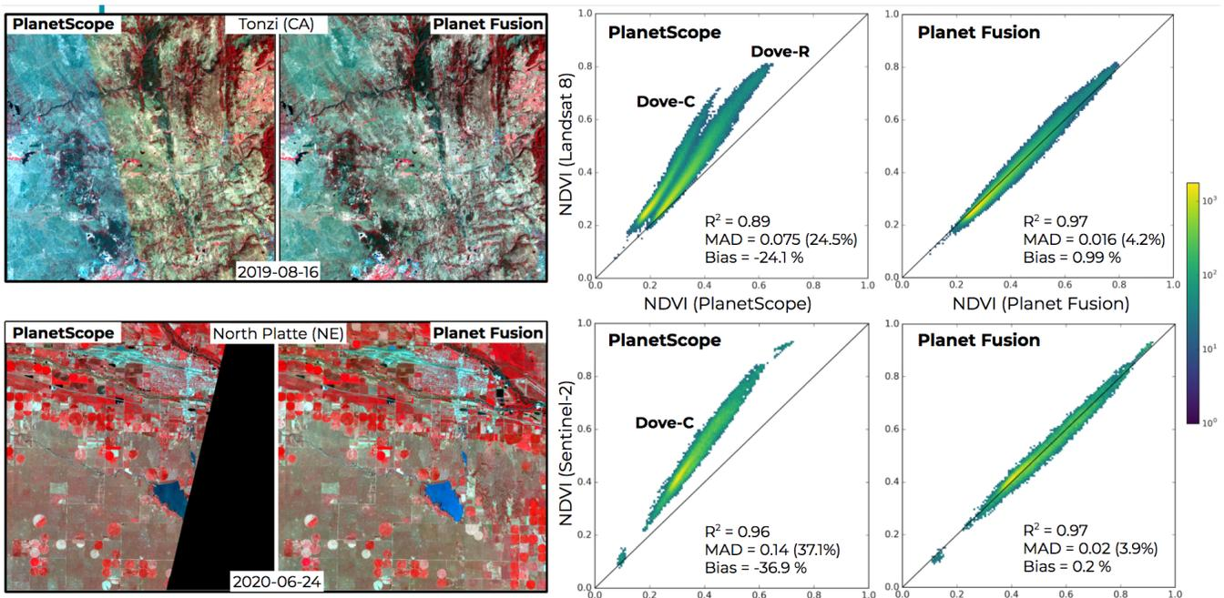
Figure 15: Real versus synthetic (gap-filled) Planet Fusion data for different observation gap intervals (false color: NIR, Red, Green)
